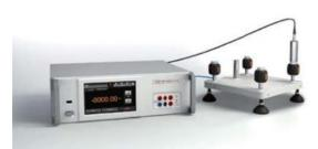
After assembly each sensor is temperature compensated over the range of 0 °C to 50 °C. The Additel 780 series can be equipped with one internal pressure sensor and one external pressure sensor. The modular design of this unit provides for interchangeability of both the internal and external sensors with other intelligent pressure modules. In addition to the Intelligant Pressure Modules.
