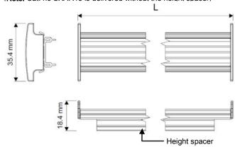
without the height spacer for mounting on DIN rails 7,5 mm depth
