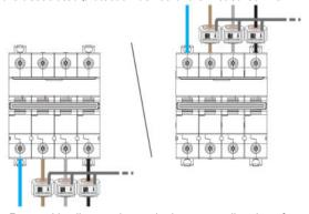
. Rogowski coils must be put in the correct direction of current flow  $(\mbox{arrow drawing on the coil}).$
