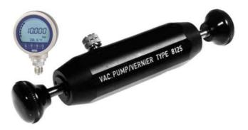
Vacuum hand pump/volume regulator 8125 is a very handy tool for the generation and the adjustment of vacuum pressures. This unit can generate vacuum pressures down to approx. – 0,75 bar. The pump's plastic casing is designed to assure a maximum grip capability and the material prevents heat transfer by e.g. hand warmth. The pump is compact, lightweight and rugged, making it ideal for field use. The simple design and quality construction ensure a long service life.
