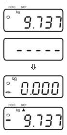
⇒ Put the test objects subsequently on the weighing plate, the respective deviation from the nominal weight is displayed with the respective sign to "+" and "-" (e.g. + 0.037 g).
