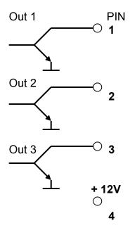
Diode connecting plug 5 pol. Typ Masei 5100 S version D
