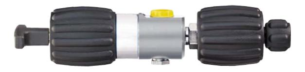
The ICP 4 pneumatic manual pressure pumps are compact, lightweight and portable calibration pumps for pressure and vacuum. Switching is controlled by a valve without the need for additional tool. The pumps allow very simple and exact operation in the pressure ranges from -0.3...4 bar
