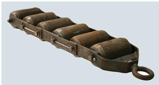
Roller test chains are used for belt scale calibration when material tests are not practical. All test chains are bushed. Minimum length is 4 feet (1.2 m).
