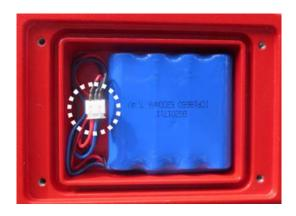
Before the first use, the rechargeable battery should be charged by connecting it to the mains power cable for at least 24 hours. The operating time of the rechargeable battery is approx. 60 hours.
