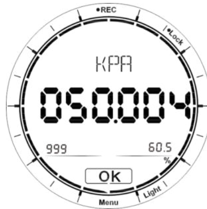
Figure 10 pressure record operation interface
