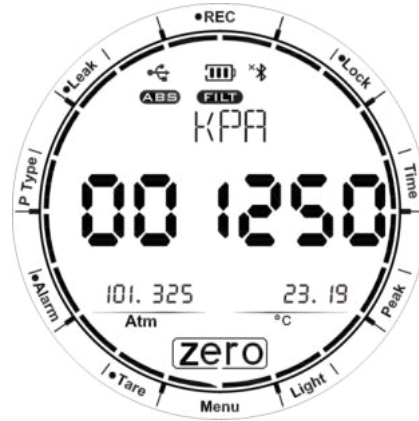
Figure 3 Main Operation Interface
