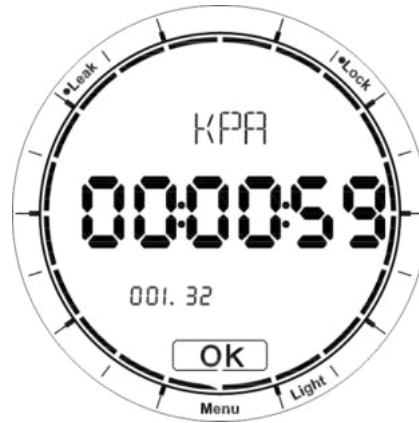
Figure7 Pressure leak test operation interface
