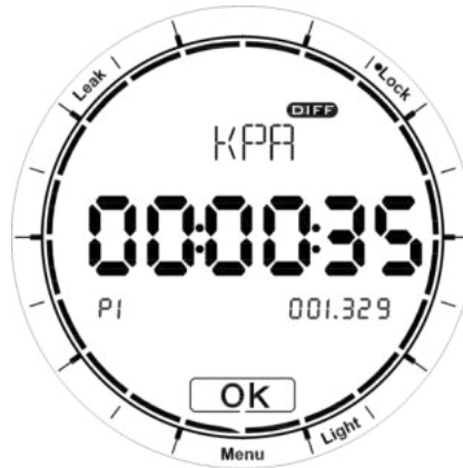
Figure 8 Pressure leak test finish interface
