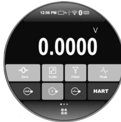
Figure 6 Electrical signal measurement function
