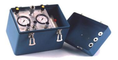
The Separator Unit Model 2255 is a complete unit for oil-free testing and calibration, normally in combination with a hydraulic Deadweight Tester. The unit contains an Oil/Gas Separator Model 8335 and a gas pressure control unit. The separator has no diaphragm between the oil and gas. The natural separation between the two media does not affect the accuracy of measurement. The level of separation can be checked through the monitoring glasses.
