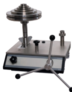
Hydraulic pressure balance, model CPB5800
