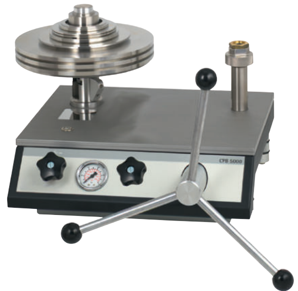
Pneumatic pressure balance, model CPB5000
