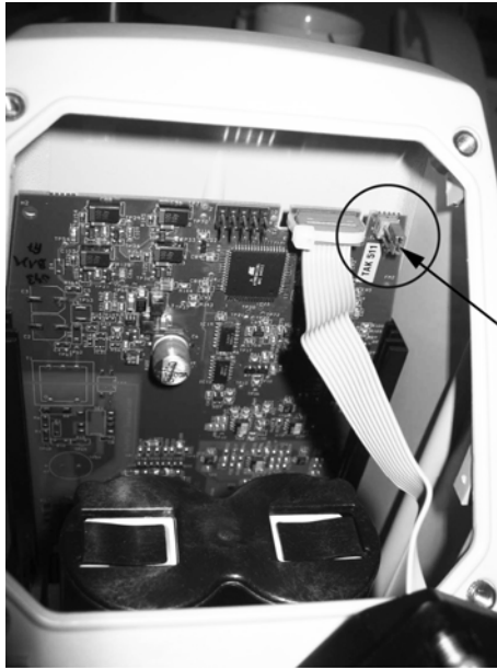
Figure 7-3 HW key behind the display (pins to the right)
