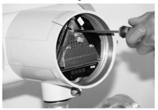
5. Change termination at the transmitter cassette by changing the position of the dip switches as below.
