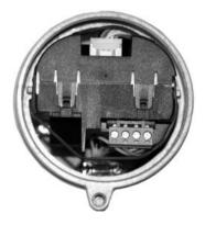
13. Assemble and tighten cable gland.
