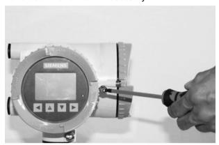
3. Carefully remove display and cable plug.
