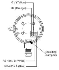
Figure 4-2 Sensor terminal compartment
