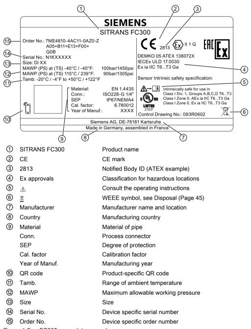
Figure 1-2 FC300 nameplate example
