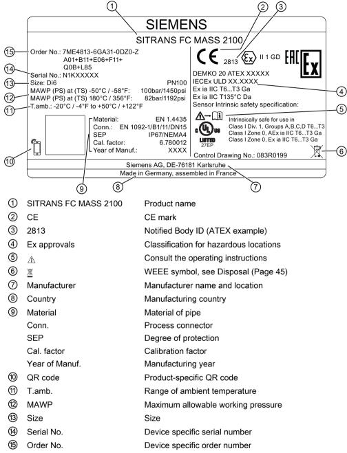
Figure 1-1 MASS 2100 nameplate example
