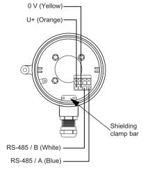
Figure 4-3 Sensor terminal compartment
