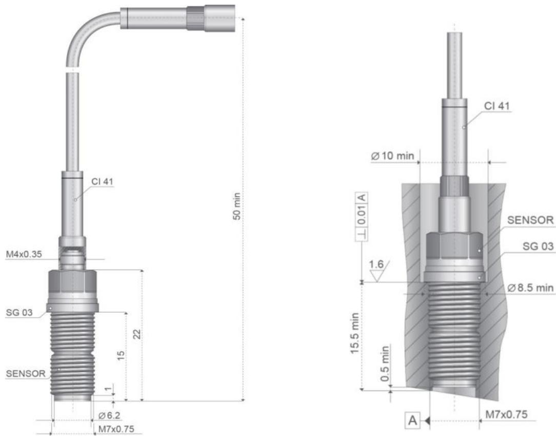
The sensor can be screwed directly into the object to be measured. The sensor rear side ( $\text{Ø } 8.45 \text{ mm}$ ) seals the sensor in the mounting hole. Rapid changes in pressure are best detected when the volume in front of the membrane is kept as small as possible.
