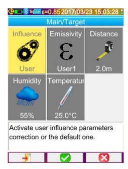
When user compensation is selected, the various parameters can be adjusted:
