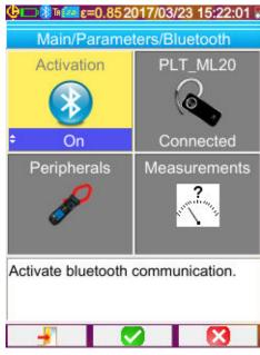
To use this function, you must first activate it from the Main/Parameters/Bluetooth menu by setting the Activation to "On" (validate the item with F2 У, to allow item entry, use Up/Down to change the value, and F2 🗹 to validate the entry).
