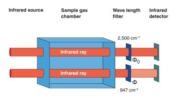
In the gas detector model GIR-10, the sucked-in air is pumped through the sample chamber. The concentration of SF<sub>6</sub> gas is determined electro-optically by means of absorption of SF<sub>6</sub> at 947cm<sup>-1</sup>. The output signal of the detector is directly proportional to the absorption of the infrared light at the specific wave number. The GIR-10 does not need consumables and is maintenance-free within the calibration cycle.
