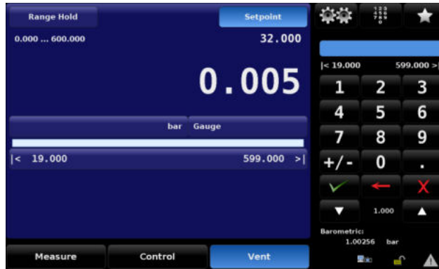
Figure 7-4 Output pressure setpoint
