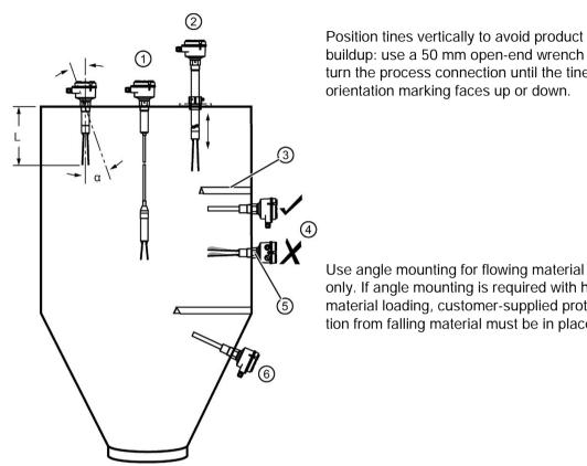
SITRANS LVS100/200 is normally mounted into the vessel top for full detection, or through the tank wall at the detection level, for full, demand, or empty detection.
