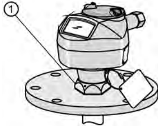
① Locking ring 1) over threaded connection; secured by three 2 mm Allen set screws
