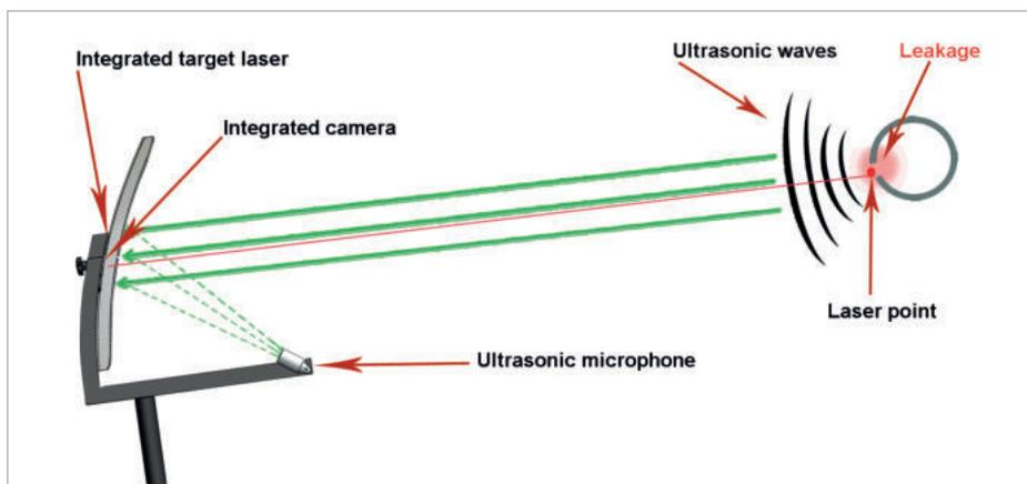
By focusing the ultrasonic waves in the parabolic mirror, even the smallest leaks of 0.8 l/min (approx. € 8 p.a.) can be located with pinpoint precision ( $\pm 15$  cm) at a distance of up to 10 to 15 m.
