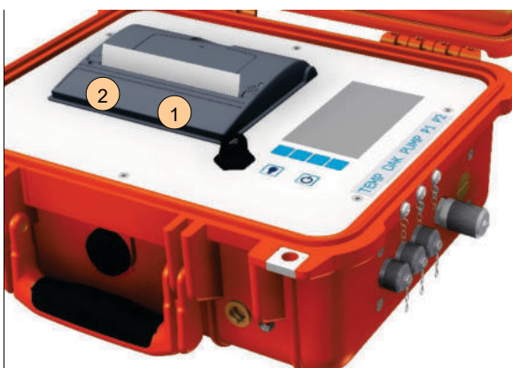
Fig. 8.4: Printer status LED and paper advance button
