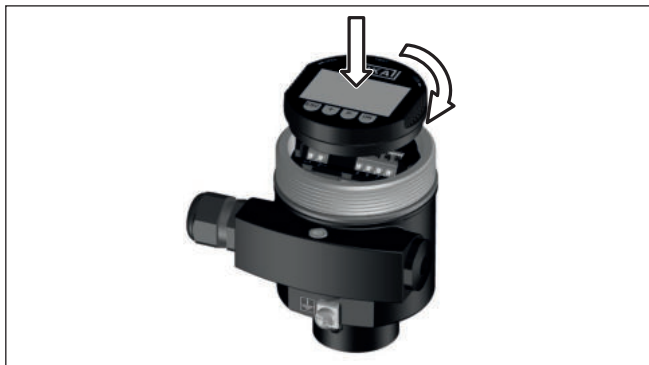
Fig. 38: Installing the display and adjustment module in the electronics compartment of the single chamber housing
