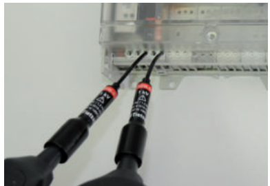
Pin prod SPB-S70 for secure testing of close contacts
