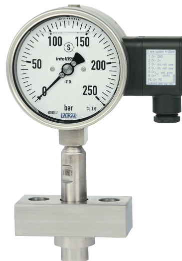
Diaphragm seal model 990.30 with directly mounted Bourdon tube pressure gauge with electrical output signal model PGT23.100
