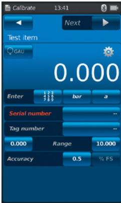
Menu screen of the operating mode “Calibration”
