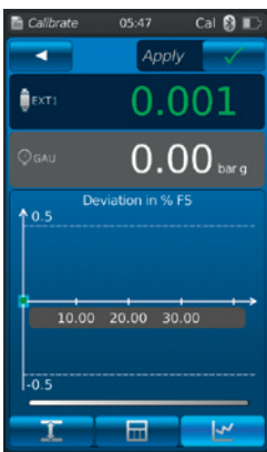
Representation of calibration results as graph
