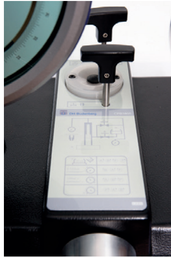
Control schematic on the CPB3800 instrument base
