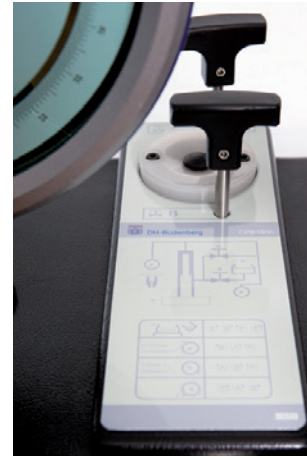
Control schematic on the CPB3800HP instrument base
