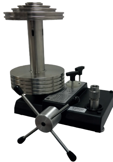
Dead-weight tester, high-pressure version, model CPB3800HP
