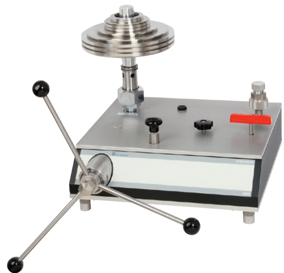
Pressure balance, high-pressure version, model CPB5000HP
