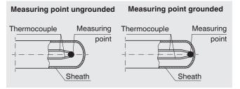
The thermocouple will be delivered as a single thermocouple with an ungrounded measuring point, unless explicitly specified otherwise.
