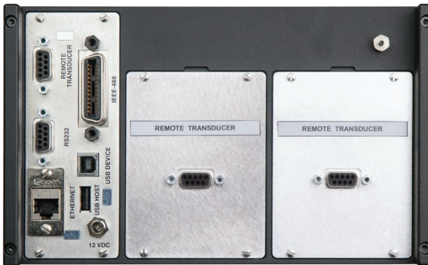
Figure 5.4 B - Two remote transducer interface connections installed
