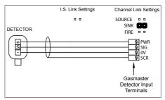
Figure 2.14 Connections for 4-20 mA 3 wire Flame detector, 4-20mA/Fire input module
