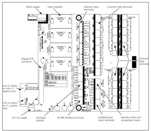
Figure 2.5 Terminal PCB layout
