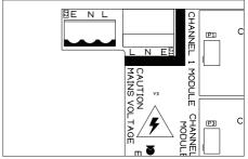
Figure 2.4 Mains connection terminals on terminal PCB
