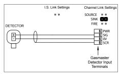
Figure 2.6 Connections for 2 wire detector 4-20mA/Fire input module
