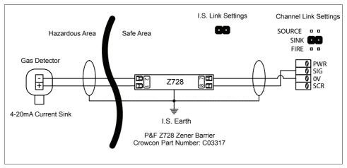
Figure 2.7 Typical connections for 2 wire I.S. detector with Zener barrier, 4-20mA/Fire input module Set channel link to SINK (see figure 2.5) and configuration to DET4-20 SINK (see Menu System Overview section, page 25 and 33. Refer to earth connection requirements on Figure 2.5, page 7
