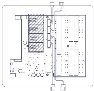
Figure 5.1 Connections for mV pellistor type detectors. mV Pellistor input module
