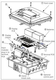
Figure 2.1 Exploded view of Gasmaster
