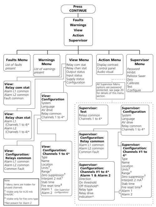
Figure 3.5 Overview of Gasmaster Menu system
