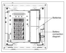
Figure 4.1 Battery replacement
