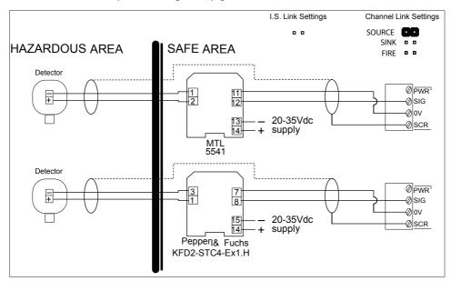
Figure 2.8 Typical connections for 2 wire 1.5. detector with Galvanic Isolator, 4-20mA/Fire input module. Set channel link to SRCE (see figure 2.5) and configuration to DET4-20 SRCE (see Menu System Overview section, page 25 and 33.
