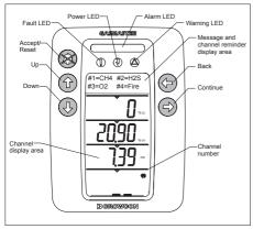
Figure 3.1 Operator Display Panel and buttons
