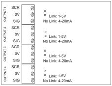
Figure 2.18 Gasmaster analogue output connection terminals
