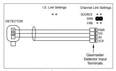
Figure 2.9 Connections for 3 wire detector 4-20mA/Fire input module
