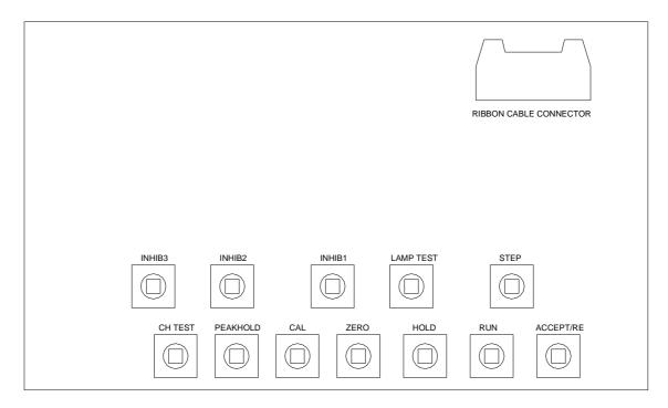
Figure 4 – Rear of Display Module
