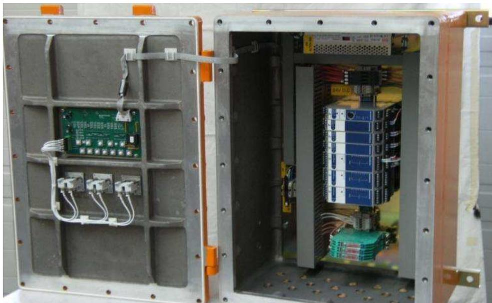
Once the brackets are attached, close the door and restrain using one fixing bolt before attempting to mount the cabinet.
