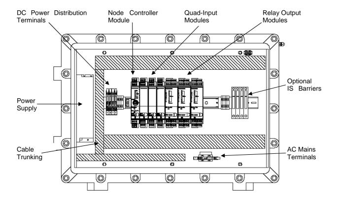
Figure 1 – System Internal View
