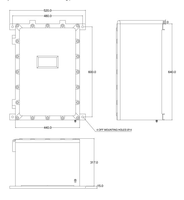
Figure 2 – System Dimensions and Mounting Detail
