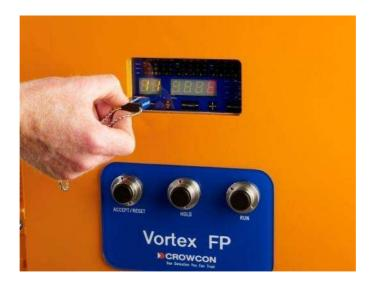
Vortex FP incorporates a Display Module which is fitted behind a window, and provides a display of detector signals and reports the current status of the system. Display functions are controlled using a Crowmag calibration tool, which should be oriented (horizontally or vertically) as indicated by the arrows on the display function fields.
