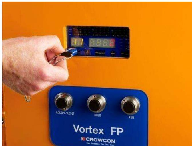
Vortex FP incorporates a Display Module which is fitted behind a window, and provides a display of detector signals and reports the current status of the system. Display functions are controlled using a Crowmag calibration tool, which should be oriented (horizontally or vertically) as indicated by the arrows on the display function fields.
