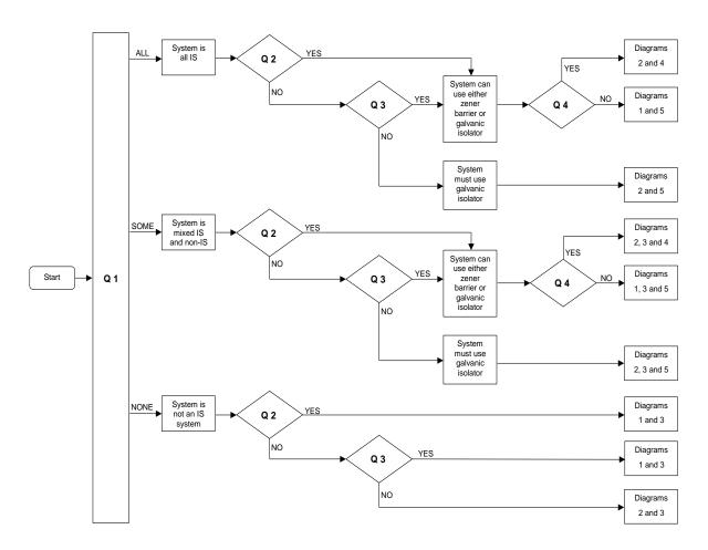
Figure 20 Decision Tree for determining Earthing Requirements
