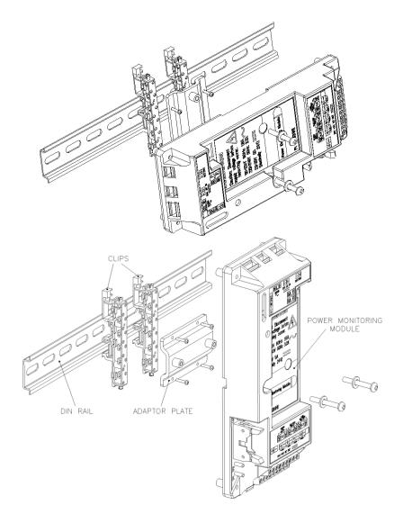
Figure 12: Alternative mountings for the Power Monitoring Module
