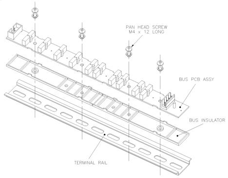
Figure 4: Bus Rail Assembly Details
