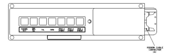
Figure 9: Back of Display Module
