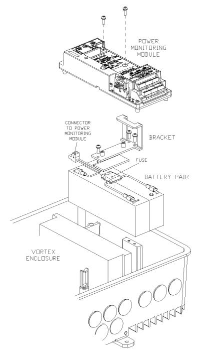
Figure 15: Removing batteries from Vortex Standard Enclosure
