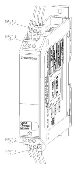
Figure 5: Quad Channel Input Module
