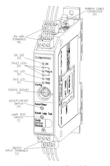
Figure 3: Node Controller Module
