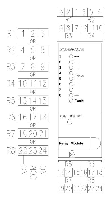
Figure 19: Wiring diagram for the Relay Output Module
