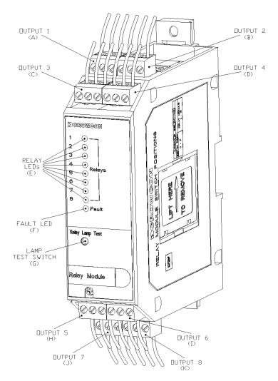
Figure 7: Relay Output Module
