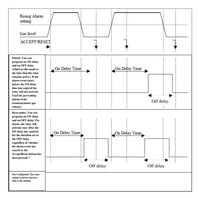
\*Note: The Reset Pulse relay function is typically used for automatic reset of latched alarms by connecting relay contacts to the 'Remote Accept/Reset' terminals on the Node Controller.
