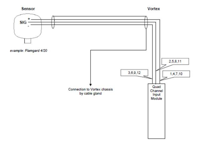
In a system with mixed IS and flameproof sensors in a hazardous area (Zone 1 or 2), the flameproof sensors can be connected as shown above providing the sensor complies with relevant standards.
