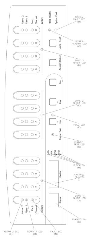
The Display Module shown is for Vortex (in its standard enclosure), Vortex Rack and Vortex panel have only minor differences in outline.
