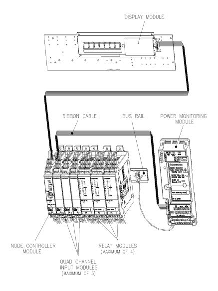
Figure 1: General Assembly of Vortex Modules
