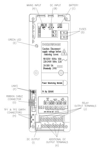
Figure 11: Power Monitoring Module
