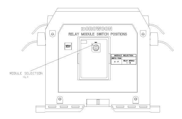
Figure 8: Relay Output Module Selection Switch
