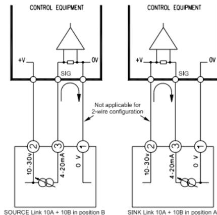
Figure 2.1 Electrical connections for 4-20 mA device
