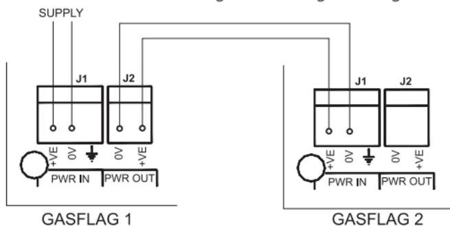
Figure 5.1 Electrical connections for daisy chaining two Gasflags
