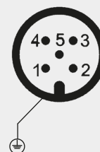
Circular connector M12 x 1, 5-pin
