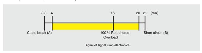
With a fixed signal level of, for example, 4 mA, the testing cycle can be triggered in every operating status upon activation of the check relais. The measurement's upper limit
