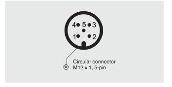
Connect the cable shield to the force transducer housing. In the case of accessory cables, the cable shield must be connected with the knurled nut and thus connected to the housing of the force transducer. When extending, only shielded and low capacitance cables should be used. The permitted maximum and minimum lengths of the cable are specified in ISO 11898-2. A high-quality connection of the shielding must also be ensured.
