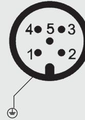
Connect the cable shield to the force transducer housing. In the case of accessory cables, the cable shield must be connected with the knurled nut and thus connected to the housing of the force transducer. When extending, only shielded and low capacitance cables should be used. The permitted maximum and minimum lengths of the cable are specified in ISO 11898-2. A high-quality connection of the shielding must also be ensured.
