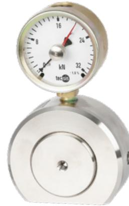
Hydraulic compression force transducer, model F1119
