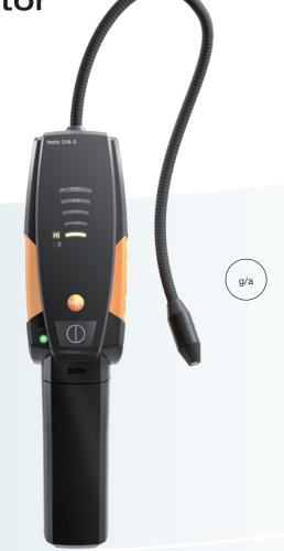
testo 316-3 is a reliable leakage detector for refrigerants which should be a part of every professional's refrigeration technology equipment. It detects even the smallest leaks thanks to its high level of sensitivity of 4 g/a, and fulfils the requirements of the F-gas regulation as well as the standards SAE J1627 and EN14624:2012.
