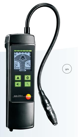
The testo 316-4 (Set 1) is a fast and reliable leakage detector for all common refrigerants. The sensor is permanently monitored and shows malfunctions or contamination in the display. The use of test leaks is thus superfluous. If dirty, the sensor can simply be cleaned, and is immediately ready for use again.
