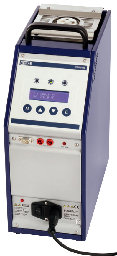
Temperature dry-well calibrator, model CTD9100-1100
