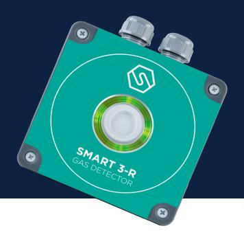
The SMART 3-R is designed for non-classified and safe areas, providing reliable detection of flammable, toxic, and refrigerant gases. It features built-in visual and audible alerts, analog 4-20 mA, digital RS485, and relay outputs, along with a multi-color LED status indicator and an internal buzzer for enhanced monitoring and safety. A handheld communicator allows for easy testing and calibration, and remote sensor capabilities add flexibility to its operation.
