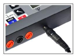
Please connect the plug of the charging component to the corresponding connector of the measuring device. **Do not use force when plugging in the plug.**
