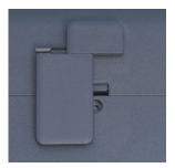
Now remove the battery cover. The unit has four AA sized batteries with a nominal voltage of 1.2V. **Please use only rechargeable NiMH batteries**. We recommend Ansmann maxE 2500mAh.Arrangement:
