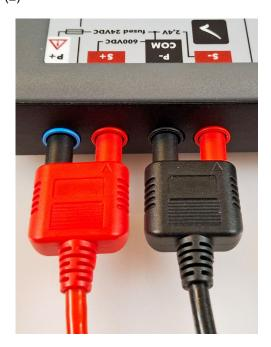
Hint: Depending on the device version, the P+ input is equipped with either a black or a blue socket. Only use the P+ input for resistance measurement at a maximum voltage of 24VDC.
