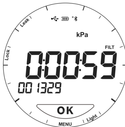
Figure 6 Pressure leak test setting interface
