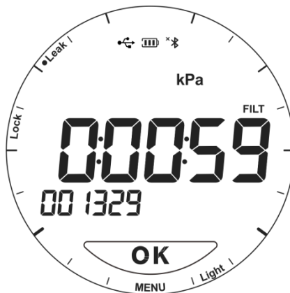
Figure7 Pressure leak test operation interface
