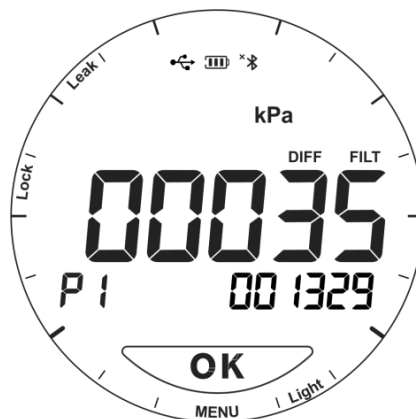
Figure 8 Pressure leak test finish interface
