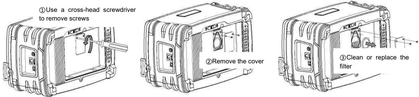
Figure 8- 1 Disassembly of the suction filter
